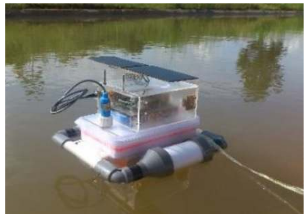
Gambar 9. Peralatan Monitoring Cemaran Air Raksa
