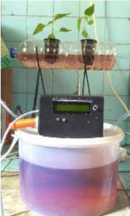
**Gambar 8.** Tampilan Prototype Sistem Hidroponik *Ebb and Flow* Otomatis
